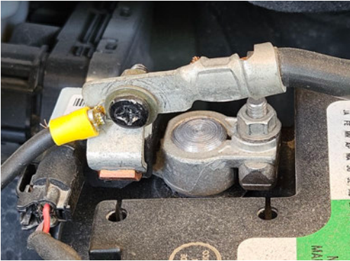
Close up of the battery current sensor with the negative lead located after the sensor.
