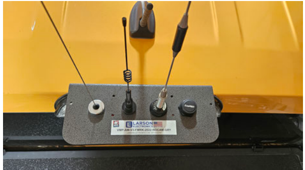
High tail light mounting plate. No drilling required.
