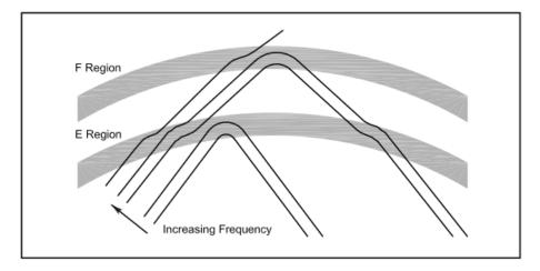
For each of the HF bands there is a Maximum Usable Frequency (MUF) and a Lowest Usable Frequency (LUF). Frequencies above the MUF escape to outer space and frequencies below the LUF are absorbed by the ionosphere. If the LUF equals or exceeds the MUF the band is closed.
